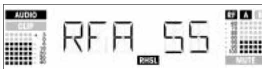
Example 2: Antenna A was active for 55% of the test period. Maximum audio level: -6 dB; minimum field strength at antenna A: -90 dB.
