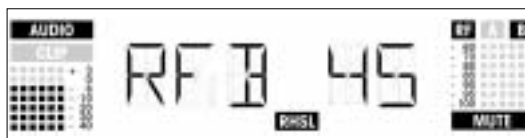
Example 3: Antenna B was active for 45% of the test period. Maximum audio level: -6 dB; minimum field strength at antenna B: less than -100 dB.
