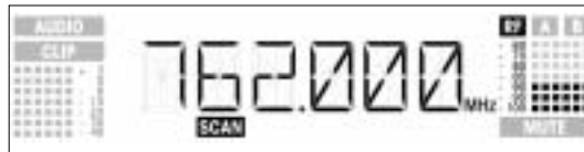
Example 1: A noise level of -90 dB has been found on the receiving frequency of 762 MHz.
