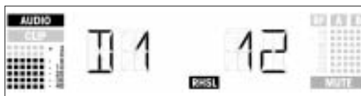
Example 1: Dropout after 12 seconds, maximum audio level: -6 dB.
